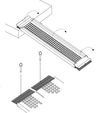
**Secure that ramp in place**: Use the 2 clevis pins supplied with the ramp to secure the ramp in place. (you will need to drill 2 holes in the step to accept the pins)
