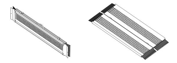
**Multifold Ramps** come in 6,7,8,10, and 12' lengths and fold in half twice producing a compact package for easy transport. Detachable lengthwise hinges allows these ramp to be transported as a single part or split in two pieces.
