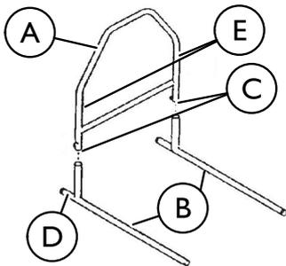
1. Install the "A" frame **A** into the floor base assembly **B** with the snap buttons **C** facing the short length **D** of the floor base.
