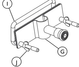
**i** Position the lower bed bracket **G** in the center of the bottom bed frame **L**. The lower bed and upper bed brackets **K** **MUST** be positioned as close to the center of the bed as possible without interfering with the bed drive shaft **M**.
