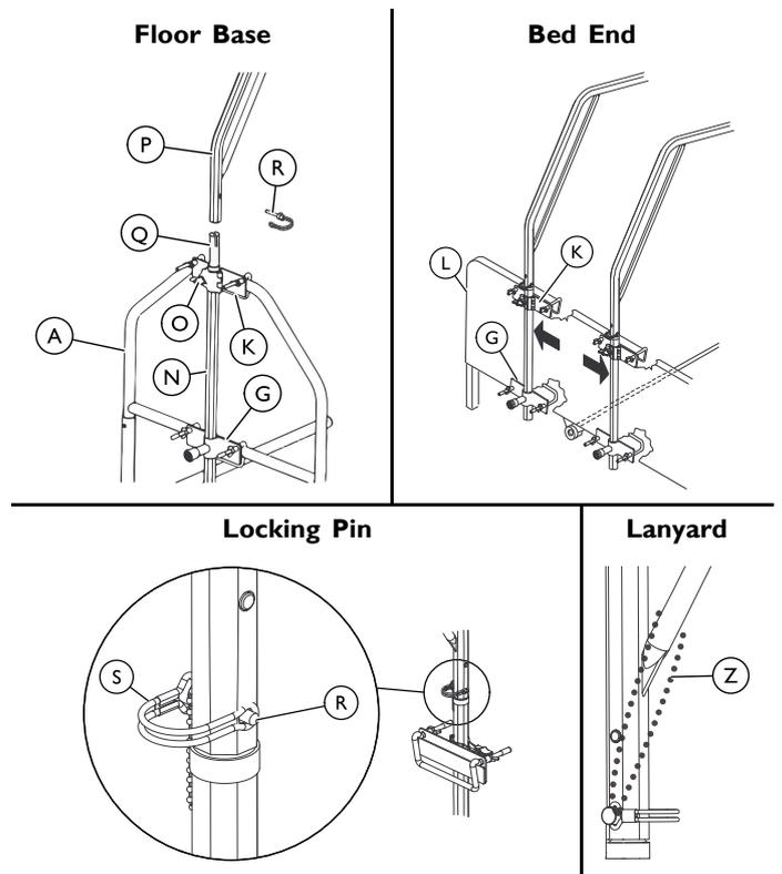
1. Install the upper bracket **K** and lower bracket **G** onto the floor base **F** or bed end **L**. Refer to Attaching Brackets to Floor Base, page 2 or Attaching Brackets to the Bed End, page 3.
