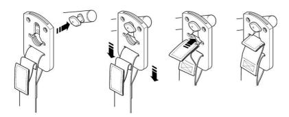
Securi3 sling attachment system. Example of installation.
