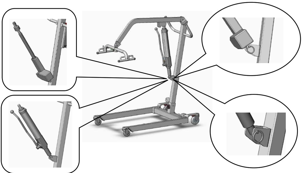
**B.** Attach the top of the Actuator to the top bracket on the Boom and insert the keeper pin and key ring.
