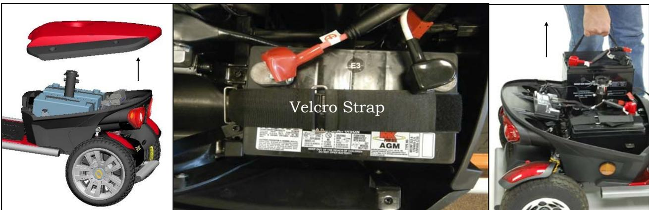
**Figure 12. Removing the Batteries**
