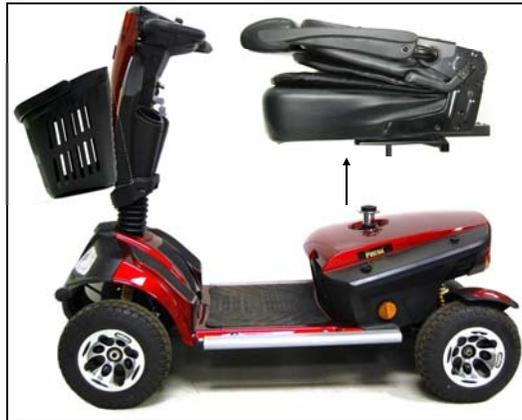
**Figure 11. Removing the Seat**
