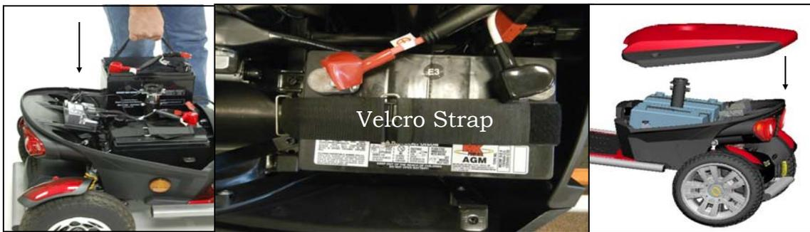
**Figure 15. Battery Installation**
