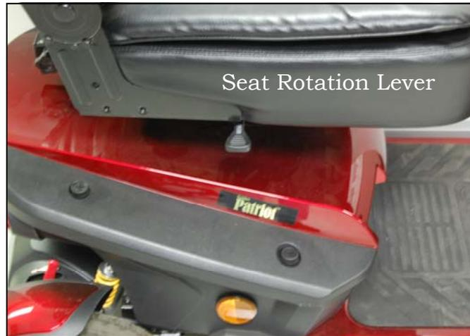
**Figure 7: Seat Rotation Adjustment**
