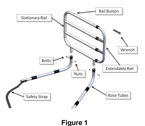
IMPORTANT: <u>The Base Tubes can be assembled 2 different ways depending on which side the bed</u> <u>the product will be used.</u> Determine which side of the bed you will be installing the product as shown in Figure 2 and then attach the Base Tubes as shown in Figure 3.
