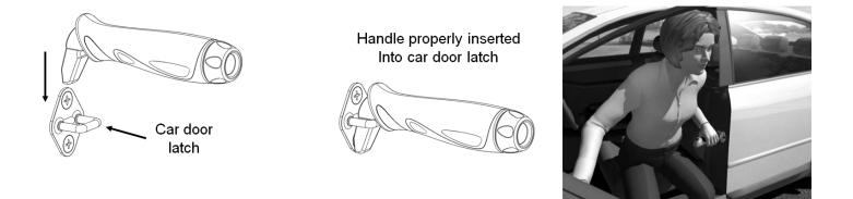
**IMPORTANT:** Do not attempt to insert the support handle into the car door latch in any other direction other than as shown in the above pictures. Failure to do so may cause injury and could possibly damage your car door latch. THE FLASHLIGHT SHOULD POINT TOWARD THE FRONT OF YOU CAR.
