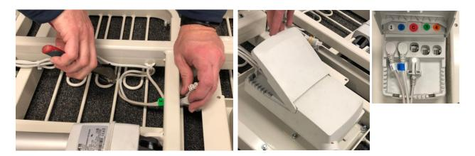
7. Turn the sleep surfaces back over, locate the head and foot labels on each section, and match them up to the correct assemblies. Then assemble them together using the bolts and nuts used to hold the bed together in the shipping form. Secure bolts tight with socket ratchet or power drill.
