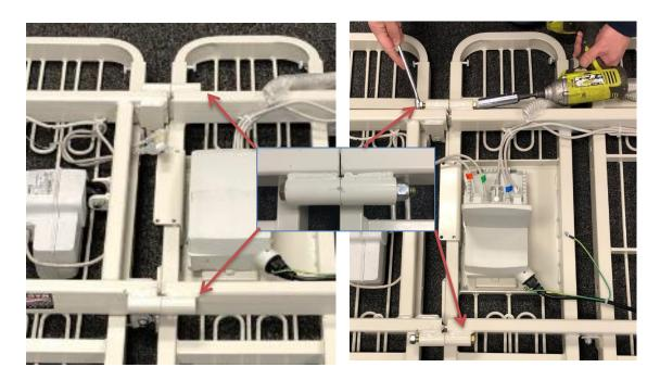
6. Find the wires labeled "3" and "4", cut the zip tie to release them then plug them into the matching ports on the control box. Route the wires in the provided slots and close the lid securely.
