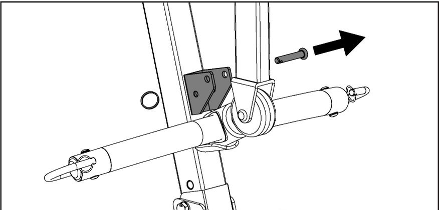
**Step 8:** Move the boom out of the way, and install the lower end of the actuator as follows
