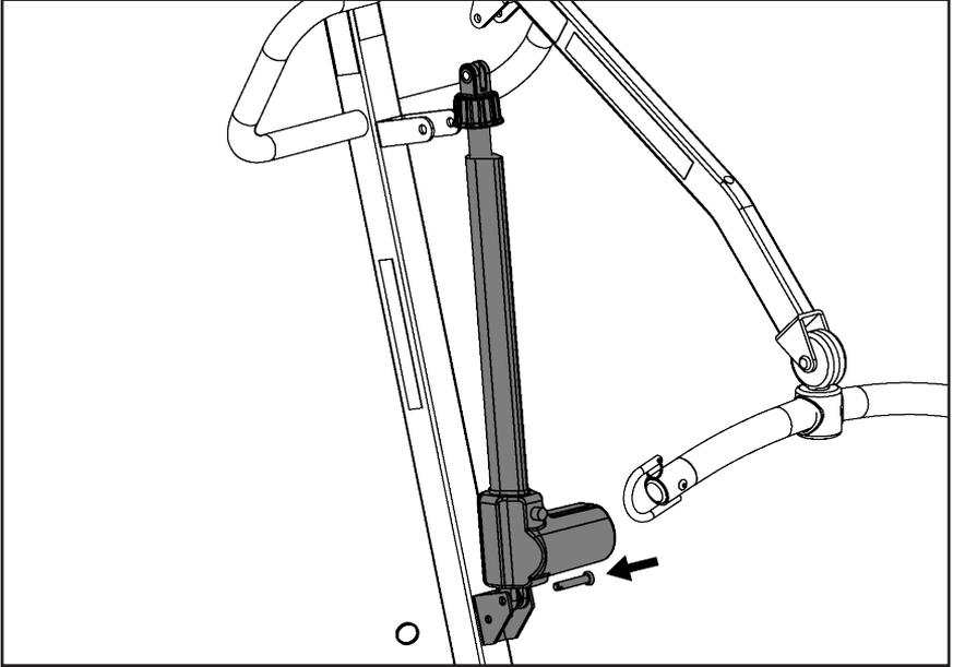
**Step 9:** Install the upper end of actuator and reinsert the quick release pin to secure it.
