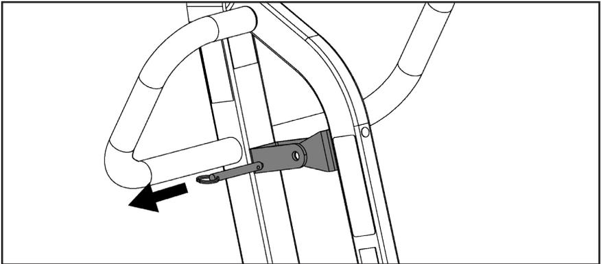
**Step 7:** Remove lower actuator pin
