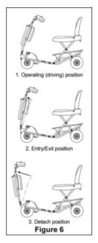
**CAUTION**: When getting in and out of the *EasyTravel* seat, step only on **CENTER** of foot platform. **DO NOT STEP ON SIDE OF FOOT PLATFORM** to avoid tipping the *EasyTravel*.
