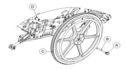
Make sure the detent pin and locking pins of the quick-release axle are fully released BEFORE operating the wheelchair.
