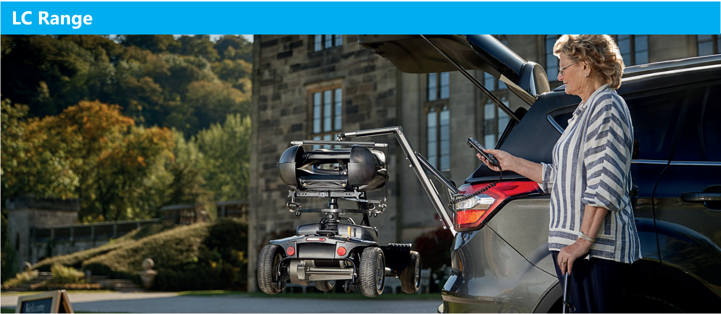
A compact hoist for scooters and powerchairs up to 220lbs that can fit a wide range of vehicles.
