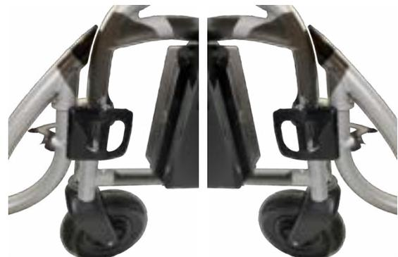
Figure 8. Install the black leg rest support into place.
