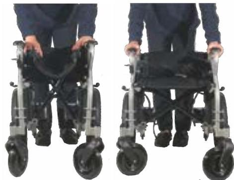
Figure 3. Lift upwards and lock into place the backrest for the seat. Ensure that the backrest is locked on each side of the wheelchair pushing the chair lock levers into position.
