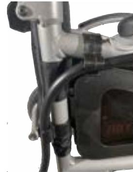
Figure 6. Connect the corresponding wires located at the rear of the wheelchair. L – L motor, R – R motor and the two red connectors together. Make sure that the wires are connected securely and to the correct corresponding wires. The connectors should snap together, making a click.
