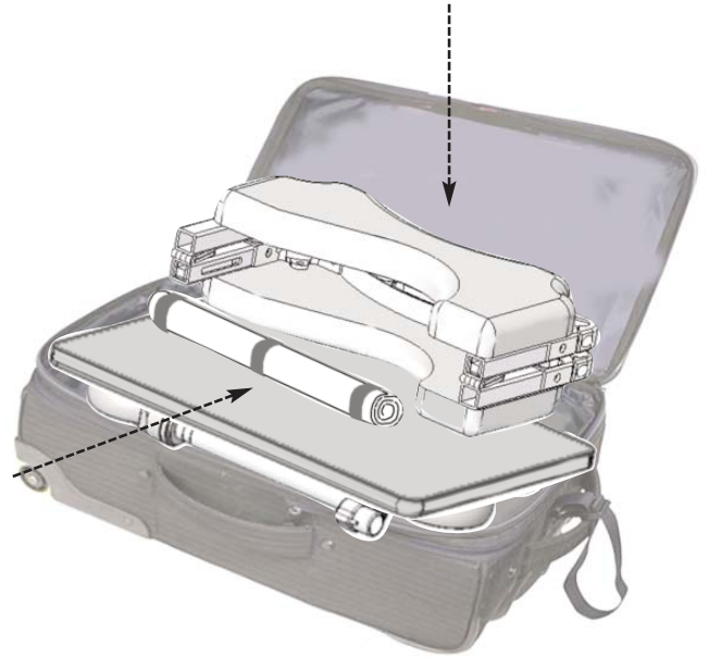
Figure B - Insert the rolled up cloth back in to the cavity of the seat frame. Then place the folded seat frame on top of the double side foam panel.
