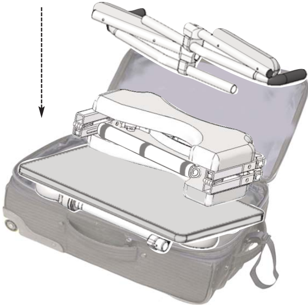
Figure C - Place the backrest posts with folded cantilever arms around the seat frame (shown here without the fabric socks). Then secure the legs, seat frame, backrest posts/arms using the black straps which are attached to the carrying case.
