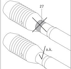
After attaching the adapter axle [22], check that it is securely held in place.
