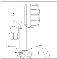
Removing the control unit
