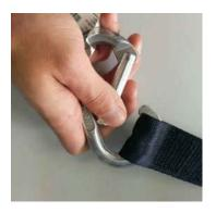
2 Install the loop of the lift strap onto the hook.
