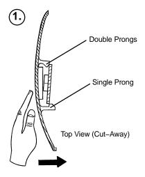
Looking through the larger of the two side cut-outs, align the cover with the axle nut or bolt head, as shown. Push down on the opposite side of the cover until the single prong engages the caster horn.
