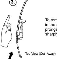
To remove the wheel cover, insert a large screwdriver into the cut–out in the side of the wheel cover and into the space between the double prongs. Pry up the cover to disengage the double prongs and push sharply upward to disengage the single prong.
