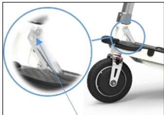
Figure 22 Steering Rod angle adjustment screws
