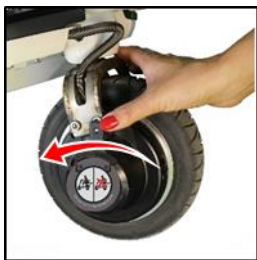
Figure 52 Securing the freewheel
