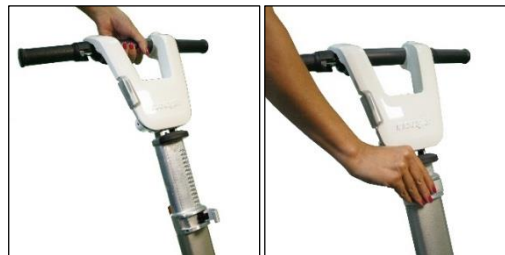
Figure 18 Driving Console height lever
