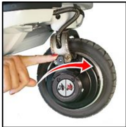
Figure 51 Releasing the freewheel
