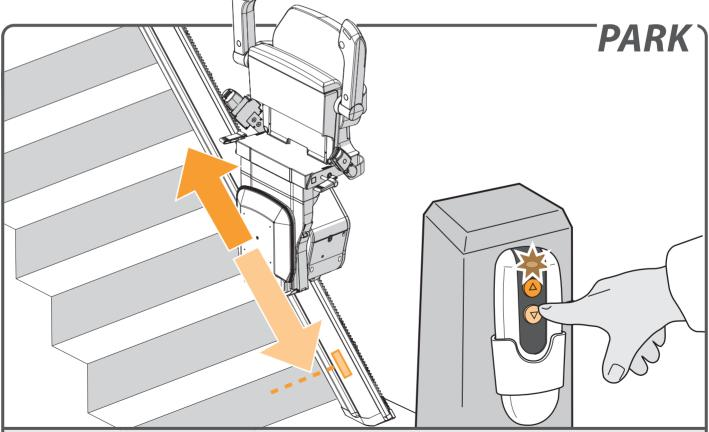
Press and hold the button on the remote control until the lift reaches a charge point. Upon arrival, the lift stops automatically and the LED on the remote control goes out.
