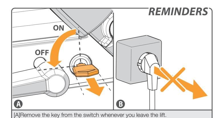
[B]Never remove the lift plug from the wall socket.
