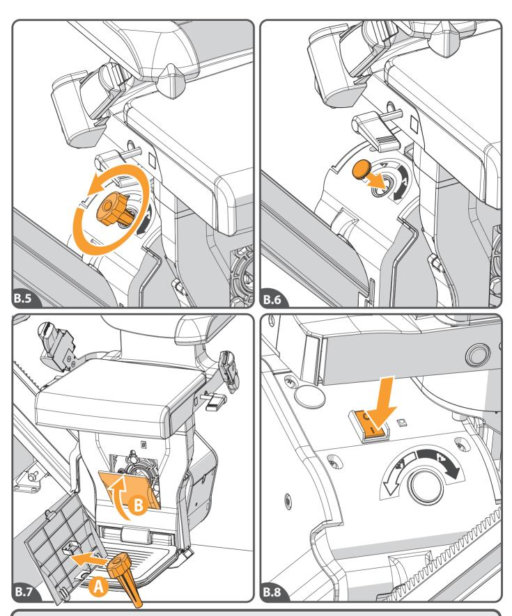
[B.5]Turn the hand winder as indicated on the winder access point. Then wind the lift in the required direction. [B.6]Replace the cap. [B.7]Replace the winder(A) and the cover{B}. [B.8]Turn on the lift.
