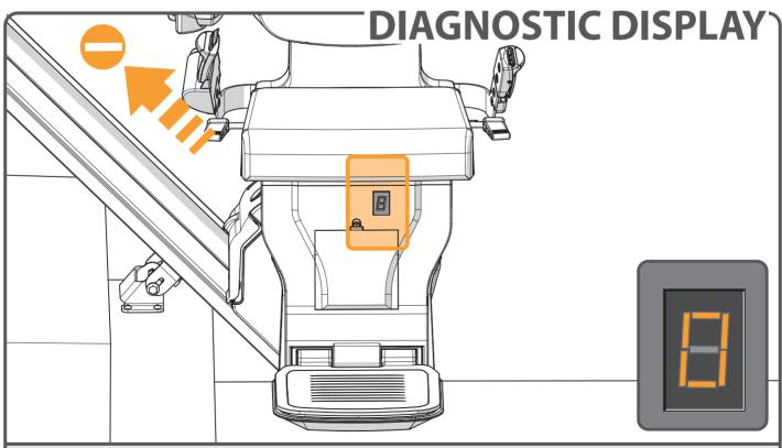
The stairlift is fitted with a diagnostic display that displays a code to help diagnose faults. Refer to APPENDIX C for an explanation of the diagnostic codes. Please inform the customer service operator of this code when reporting any fault.
