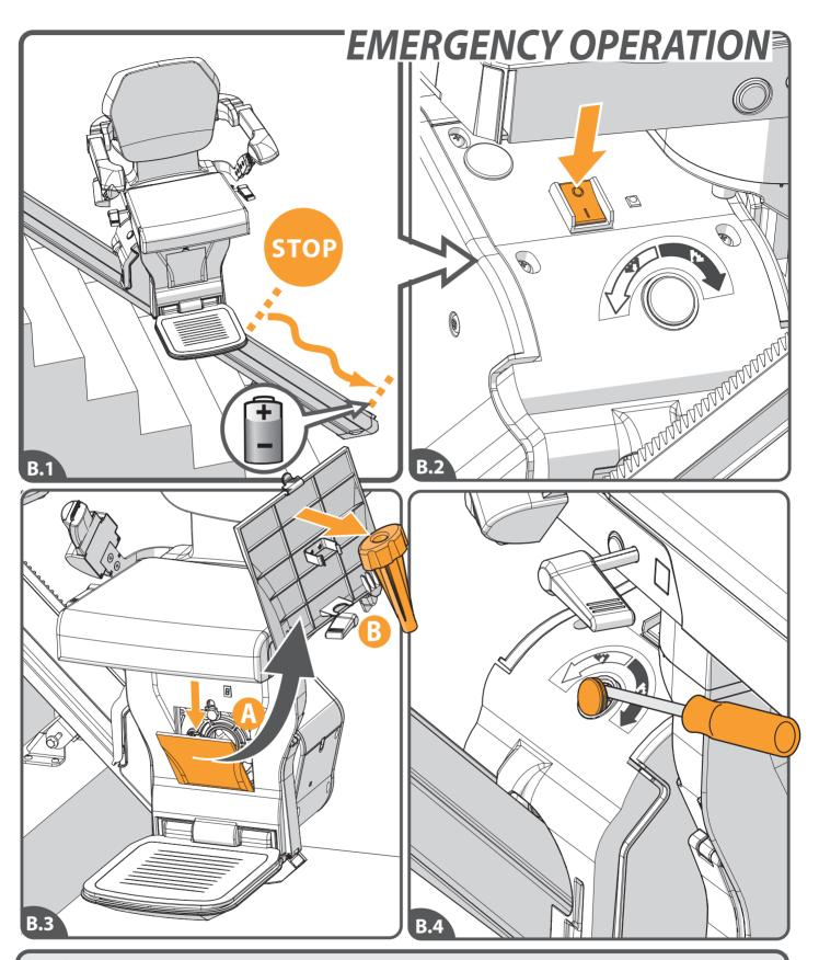
[B.1] When the stairlift stops unexpectedly and no longer moves any further, the hand winder can be used to move the lift to a charging point. [B.2]Turn off the lift. [B.3]Open the cover in the front plate of the chassis, by pressing the tab at the top of the cover{A}. Take the hand winder from the cover{B}. [B.4]Remove the cap from the unit with a screwdriver.
