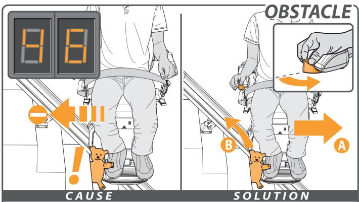
Problem: the lift travels in one direction only and the display shows a "4/6".
