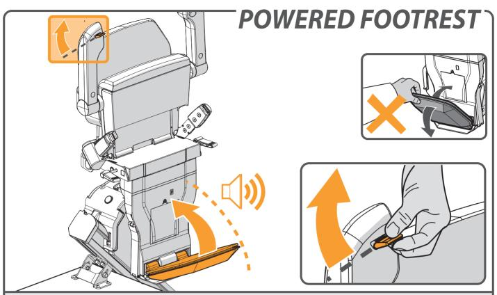
To operate a POWERED FOOTREST move the switch under the armrest. The stairlift should beep whilst folding the footrest.
