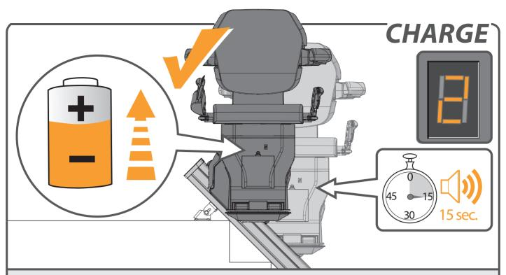
There are charge points for recharging the lift's batteries at the top and bottom of the rail (there may be additional charge points). If the lift is not in the correct position at the charge point, the lift beeps for 15 seconds and the display shows a "2". The lift does not work if the batteries are flat.
