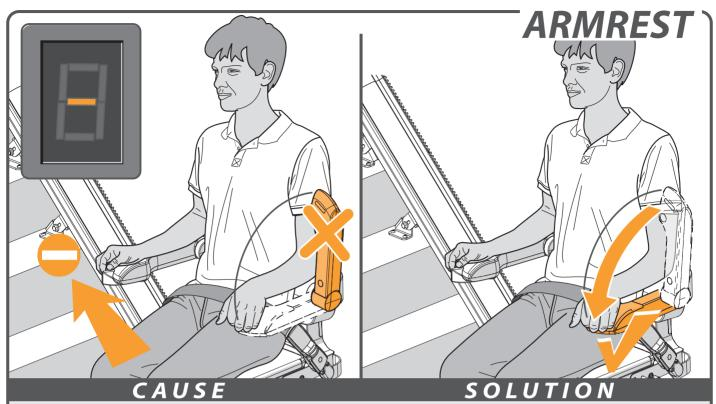
Problem: the lift does not travel in either direction and the display shows a "-".
