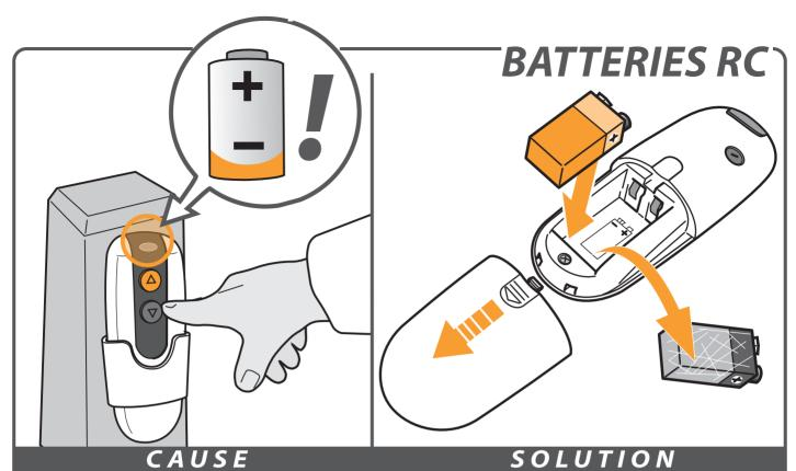
**Problem:** the lift does not travel in either direction and the LED on the remote control does not light up when the remote control is operated.
