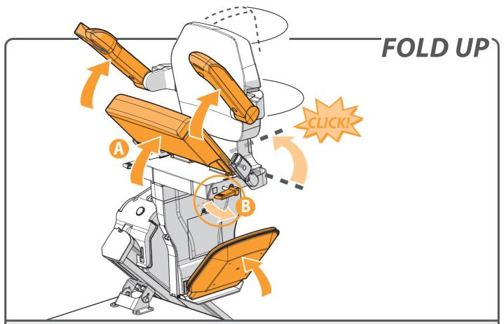
Fold up the armrests and seat {A}. Push the handle, located to the left or right under the seat, downwards {B}. Swivel the seat until you hear a 'click'. The seat is now in the locked position.
