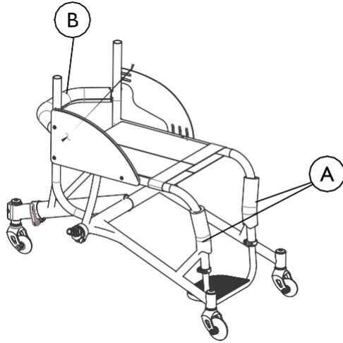
Foam pieces covered in nylon wrapping the front and rear frames and fastened with hook and loop fasteners.
