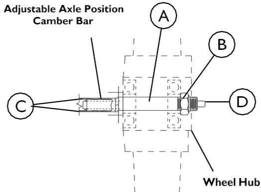
1. Remove rear wheel and quick-release axle A from the wheelchair.
