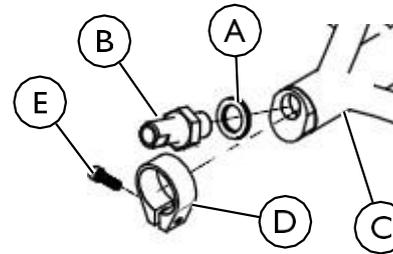
To prevent play in rear wheels, install the rear wheel bolt securing lock washer system.
