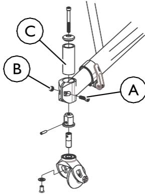
1. Loosen mounting screw A and locknut B in the side of the clamp.
