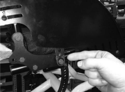
3. Insert the mounting screws A into the wheelchair frame D and back post E and secure with locking washers C and locknuts B.
