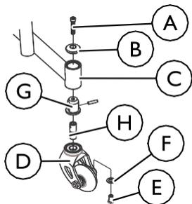
1. Place the empty wheelchair upside down so the bottom of the front fork is easily accessible.
