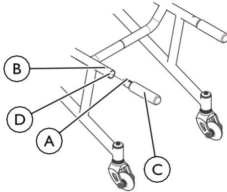
1. Facing the rear of the wheelchair, align the locking pin A with the hole on the wheelchair frame B.
