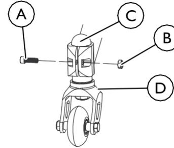
1. Loosen mounting screw A and locknut B in clamp.
