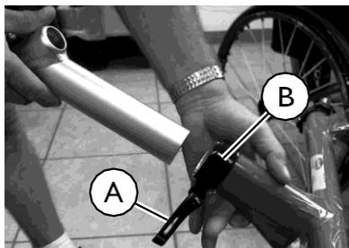
1. Release and loosen the quick release lever A attached to the anti-tip clamp B.
