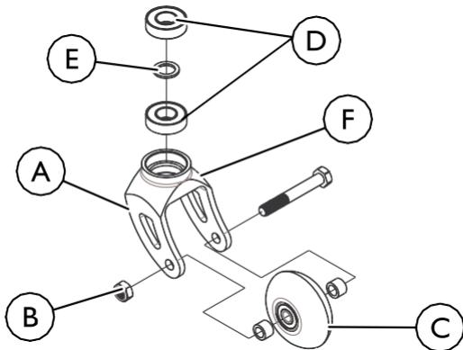
1. Place the empty wheelchair upside down so the bottom of the front fork A is easily accessible.
