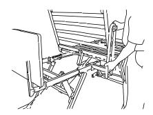
I. Raise the head section to expose the bed frame.
