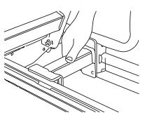
Position the Assist Bar bracket over the mounting tab on the frame.
