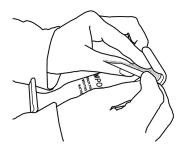
Position the hook and loop strip inside the cupped part of the pendant holster.
