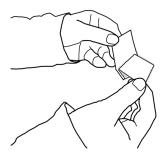
Peel the backing from the supplied hook and loop strip. (P/N PNDNT—V—LOOP).
