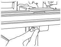
1. Insert the  $5/16-18 \times 3/4$  Carriage Screw through the back of the frame-tab mounting hole.
