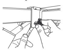
3. Tighten the cap screw with a half inch wrench while holding the knob with your other hand. Repeat for the other side.
