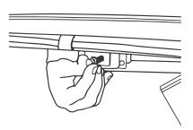
2. Place cap screw with washer through the back of the lower round hole in the side bar mounting bracket.
