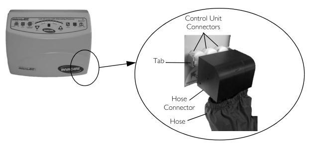
FIGURE 2.2 Connecting the Hose
