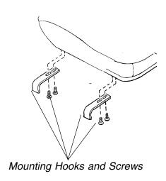
FIGURE 1 - ATTACHING / ADJUSTING THE CUSHION/BASE MOUNTING HOOKS TO THE BASE
