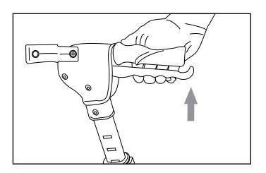
Push down on brake handle to lock the brake into PARK.
