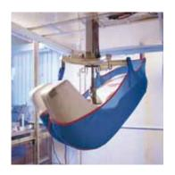
To ensure maximum safety and protection, every single sling we produce is hand tested in a specially constructed test rig. Our slings are load tested at 1.25 the maximum safe working load – over and above the formal testing requirements.
