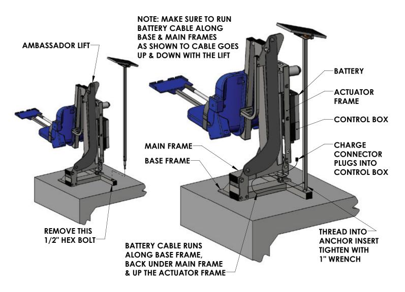
To install the Solar Charger on a Ambassador lift;
