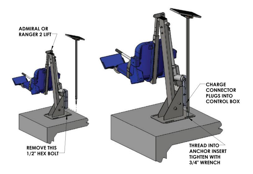
To install the Solar Charger on a Admiral or Ranger 2 lift;
