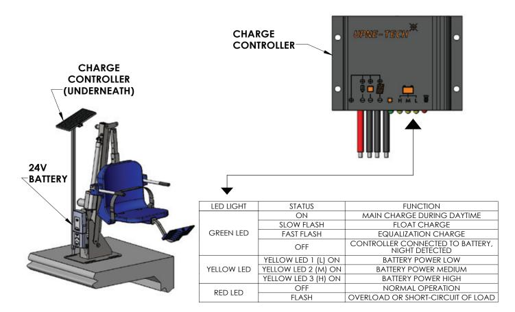
Once the solar charger has been installed and both the control box and battery have been plugged in, and there is sufficient daylight, the 24V Solar Charger will turn on and start trickle-charging the battery. Without both the control box and battery being plugged in, the 24V Solar Charger will be off and will remain off until both components are plugged in.
