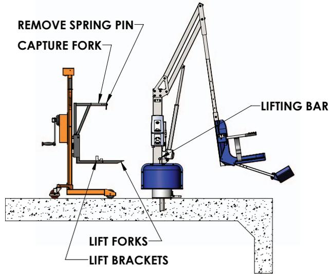
**STEP 2:** Roll the cart into position until the capture fork is around the mast and the lift brackets are under the lift bar. Replace the spring pin to hold the lift in place. See diagram to the right.
