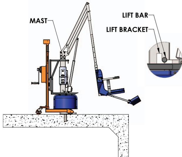
**STEP 3:** Turn the select knob clockwise to put the cart in "lift" mode. Turn the winch handle clockwise to raise the lift up and out of the anchor. If the lift won't move, shake the mast to loosen it in the anchor and turn the handle until the lift comes out of the anchor. Raise the lift until the stem is an inch or two above the floor. The lift is now ready for transportation. See diagram to the right.
