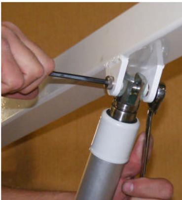
Remove the shipping strap and all packing from the **LINEAR ACTUATOR**. Connect the **LIFTING ARM** between the **MAST** and the **LINEAR ACTUATOR** as shown in the figure above. Tighten **NYLOCK NUTS (2)** until snug as shown in **PHOTO 2**. **DO NOT OVER TIGHTEN!**
